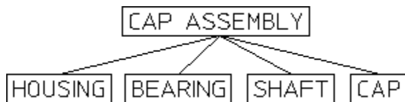
Figure 213. Cap Bearing Parts Structure
