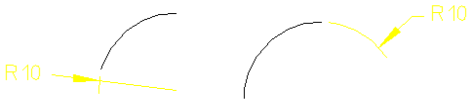
Figure 95. Dimensioning Radii with and without a Centerline
