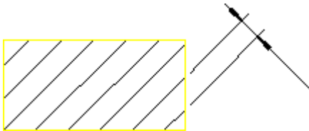
Figure 144. Hatch Line Distance
