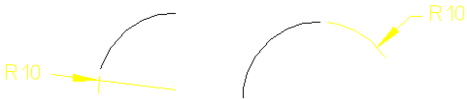
Figure 99. Dimensioning Radii with and without a Centerline
