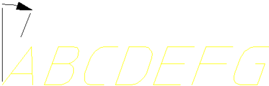
Figure 153. Text with a 15° Slant
