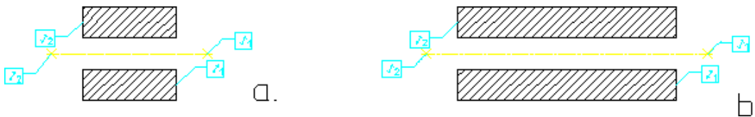
Figure 9. Distance Constraints to Control Line Length
