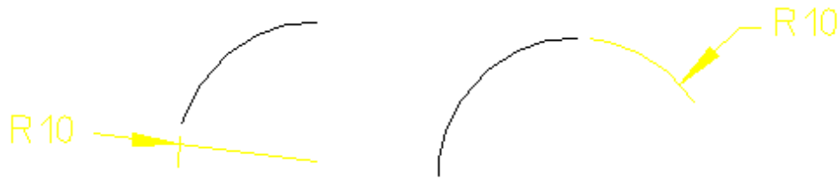
Figure 95. Dimensioning Radii with and without a Centerline
