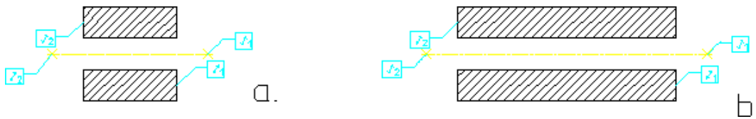
Figure 211. Distance Constraints to Control Line Length
