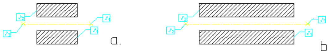
Figure 8. Distance Constraints to Control Line Length
