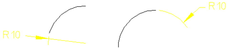
Figure 95. Dimensioning Radii with and without a Centerline
