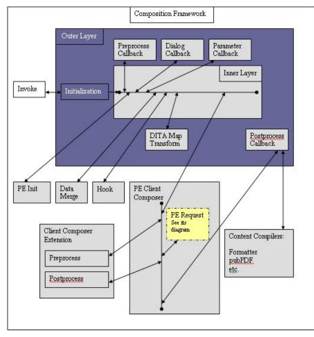
The following diagram illustrates the publishing framework processing performed on the client in preparation for sending a publishing request to the Arbortext PE server.
