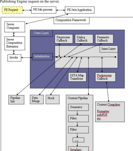
The following diagram illustrates the publishing framework processing of an Arbortext Publishing Engine request on the server.
