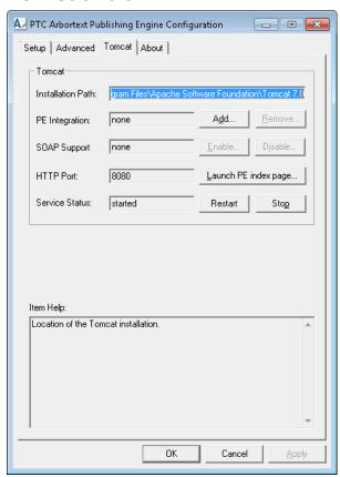
The **Tomcat** tab has a **Tomcat** group box which displays the Tomcat installation path, whether SOAP is enabled, the HTTP port Tomcat monitors, and whether the Tomcat service is stopped or started. You can add or remove the automatic integration between this installation of Arbortext Publishing Engine and Tomcat.
