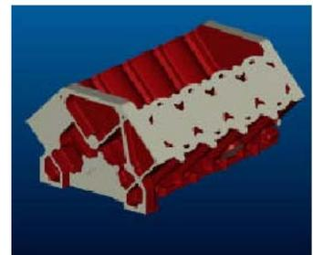
*The "as cast" model, created by temporarily removing some design content.*
