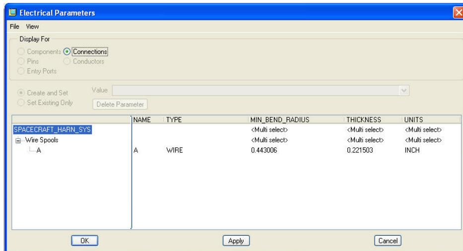
Fill out the cells for minimum bend radius and thickness. Additional parameters can be added to the spools by selecting **View, Columns** from the dialog box's pull down menus. This will bring up a dialog box to select many different electrical parameters or create user defined parameters. Add or create parameters as needed.
