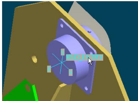
Multiple coordinate systems can be selected by holding down the <ctrl> key. Once all the coordinate systems are selected, select OK or use the middle mouse button to accept the coordinate systems selected. If desired, enter in an internal length for the ports. This length will be added to the overall length of any wire or cable routed to the port. This allows the user to create a coordinate system at the edge of the part and not inside the part where the wire will terminate.
