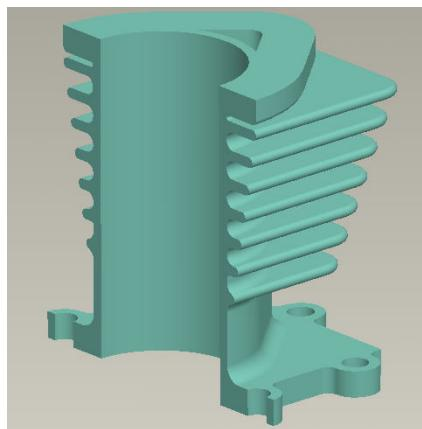
The final type of part level simplified rep we'll look at is the surfaces simplified rep. This type of rep allows the user to select a set of surfaces to be displayed for the part instead of the entire volume. These types of reps are great to use as substitutions in an assembly level simplified rep. A user can create a surfaces part level simplified rep that only contains the mating or critical surfaces of the model and substitute that rep to simplify a higher level assembly.
