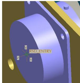
This green target is the “from” point for the route. Notice that the route option is changed to Free in the *Cbl Route* menu. This routing option allows the user to mouse pick a point on any surface to route the cable. Select a couple points for routing on any surface. Experiment with other routing options to see how easy it is to route wires and cables.
