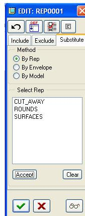
Choose the desired simplified rep and select the Accept button. The rep name should show up in the model tree next to the part name. Select the green check mark to create the rep. Multiple assembly level simplified reps can be created that reference different part level simplified reps through this substitution technique. A couple examples are shown below.
