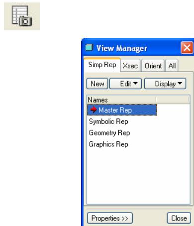
Select the Simp Rep tab near the top of the dialog box. By default, there will be four reps that already exist in the model as shown above. These reps are the master rep, symbolic rep, geometry rep, and graphics rep. These are simplified representations that are created automatically when saving a part file. Refer to PTC help for a description of each of these reps.
