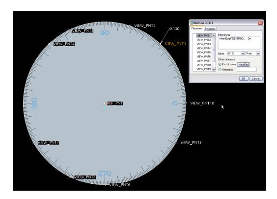
20. Create a new drawing and place the Visibility Assembly study. Use the TOP view to display the newly created line of sight indicators. Hide any excess curves as needed.
