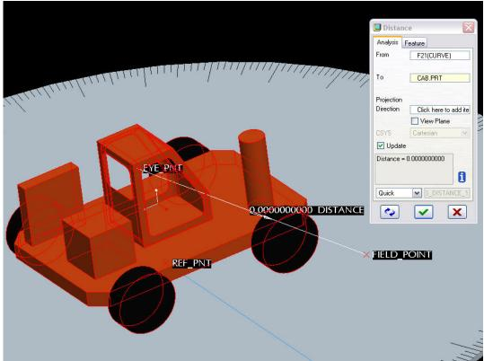
• Change the Analysis type to "Feature" and click the Green Checkbox to complete the feature.
