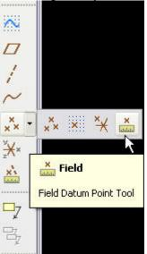
5. Place the Field Point on the top surface of the **Ground.prt**. Location of the field point on the surface is not critical. Rename the newly created point "FIELD\_POINT" to help differentiate from any existing points in the assembly.
