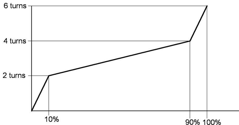
In the graph above, the first two and last two turns are completed in just 10% of the length of the spring each. The middle two turns take up the remaining 80%. This is similar to what we want our spring to do.
