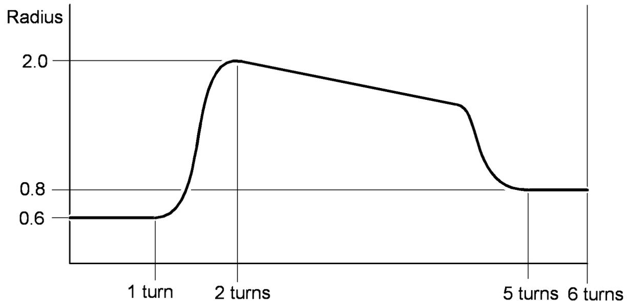
In the graph above, notice how we’re taking what we can visually see with the spring and turning it into data for our model: For one turn the radius is .6, at 2 turns the radius is 2.0, the radius decreases linearly and then transitions to be .8 at 5 turns.
