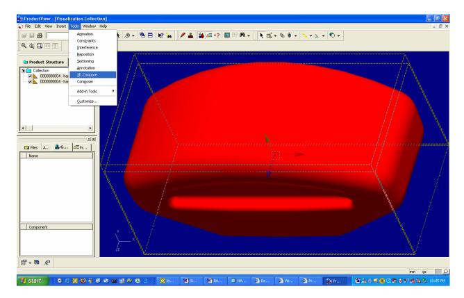
Now we are ready to run the 3-D compare. Click the run comparison icon at the bottom. Then when the results are complete then you can toggle the display.
