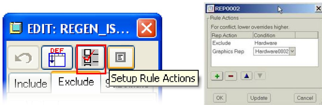
In this context it will be displayed as the Rule Editor. This will automate the filtering process with your search criteria continuously updating based on changes to the assembly. There is no need to re-create the rules or re-run your search. They can also be combined (explained later).
