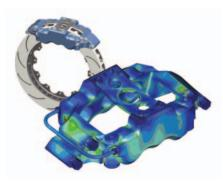
Pro/ENGINEER Mechanica enables validation of designs such as this model of a brake, and reduces the number of physical prototypes needed.
